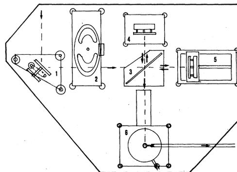
FIG. 1. Sketch of the infrared airborne radiometer. (1) Wobbling mirror, (2) chopper for absolute measurements, (3) beam splitter, (4) fixed mirror, (5) moving mirror, (6) liquid helium bolometer, and (7) pumping line for liquid helium.
