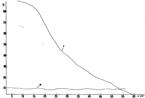
FIG. 4. Transmittance and reflectance of the airborne polyethylene window. No difference has been found before and after exposure to solar UV radiation, although the color changed significantly in the visible.
