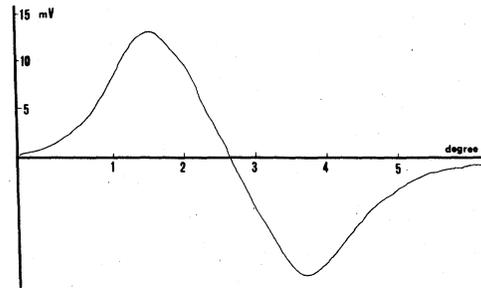
FIG. 3. Typical sun transit showing the angular response of the instrument for a  $0.5^\circ$  source.
