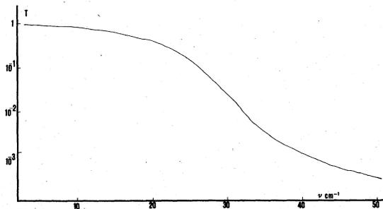
FIG. 2. Transmittance of the filters employed in the present experiment. The responsivity of the bolometer is almost flat up to 1.5 mm of wavelength.
