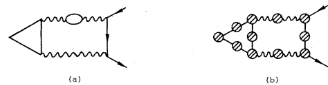
FIG. 4. (a) A photon self-energy insertion from the radiative corrections to Fig. 2. (b) The full set of corrections. The shaded blobs are renormalized propagators and vertices.
