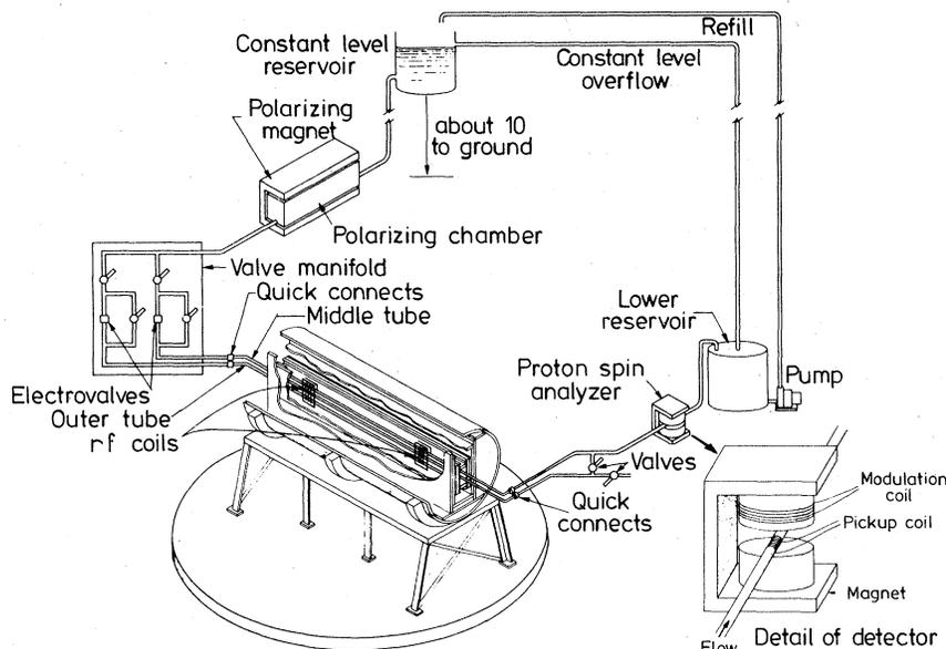
FIG. 2. Schematic view of spectrometer with detail of proton polarization and detection equipment.
