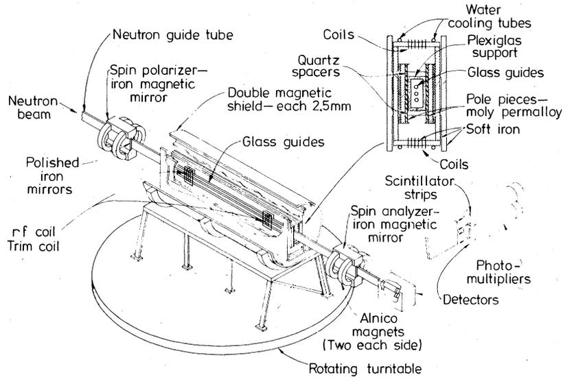
FIG. 1. Schematic view of spectrometer with detail of neutron polarization and detection equipment.
