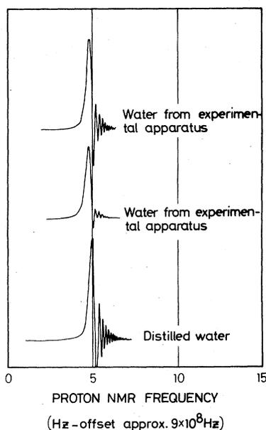
FIG. 6. Comparison between NMR signal from experimental water and distilled water. Vertical scale in arbitrary units.
