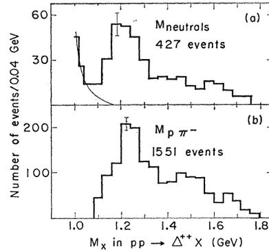
FIG. 1. Effective-mass distributions of  $X$  in  $pp \rightarrow \Delta^{++}X$  for  $|t| < 0.2 \text{ GeV}^2$  at 6.6 GeV/c. The  $\Delta^{++}$  selection is 1.14–1.30 GeV. (a)  $X =$  neutrals; (b)  $X = p\pi^-$ .
