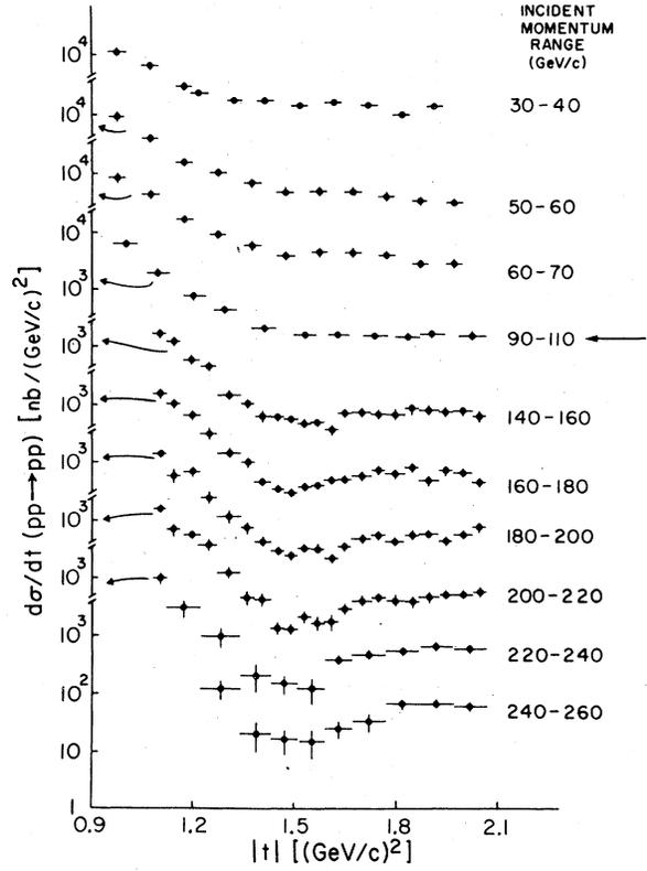
FIG. 2. Differential cross sections for proton-proton elastic scattering from 30 to 250 GeV/c, reproduced from Fig. 3 of Ref. 15.
