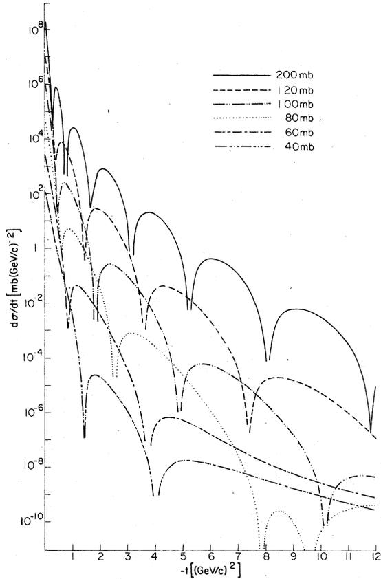
FIG. 1. Differential cross sections for proton-proton elastic scattering computed from the geometrical model for  $\sigma_T=40, 60, 80, 100, 120,$  and  $200$  mb. The vertical scale shown is for  $\sigma_T=40$  mb. The other curves are displaced from each other by a factor of 10.
