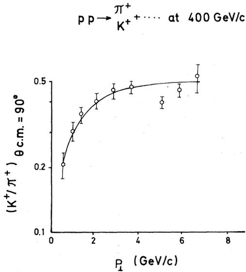
FIG. 5. Plot of  $K^+/\pi^+$  ratio vs  $P_{\perp}$  of a large- $P_{\perp}$  experiment at 400 GeV/c by the Chicago-Princeton group, Ref. 5. The solid curve is the fit to the data using a Bose-type distribution, Eq. (8) assuming the same  $T$  for  $K^+$  and  $\pi^+$ . The least-squares fit yields  $T=152 \pm 8$  MeV.
