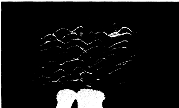
FIG. 3. Typical oscilloscope traces, including that for event A. The pulses are negative (i.e., anode pulses). Event A is the sixth one down. The top two events are multiparticle events and the next three are single-particle events all with \beta > 0.59 . The seventh and eighth events are multiparticle, and the three superimposed at the bottom not analyzable. This 23-hour time exposure was taken in May 1977.
