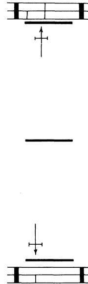
FIG. 4. Spark-chamber trajectories for event A. The arrows indicate the predicted spark positions (with their accuracies) according to the timing measurements as discussed in the text. There is an extra (out-of-geometry) spark in the top chamber. Also shown are the top, bottom, and center scintillators.
