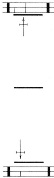
FIG. 4. Spark-chamber trajectories for event A. The arrows indicate the predicted spark positions (with their accuracies) according to the timing measurements as discussed in the text. There is an extra (out-of-geometry) spark in the top chamber. Also shown are the top, bottom, and center scintillators.
