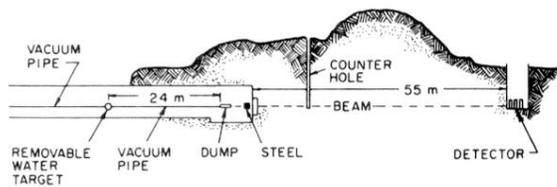
FIG. 2. Schematic of the SLAC beam-dump experiment showing the location of the detector and shielding in relation to the end station A beam dump.
