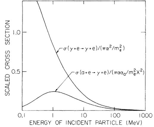
FIG. 1. The "Compton" scattering cross section for axions and photons. The axion-induced scattering cross section is enhanced in the graph by a factor  $(\alpha/\alpha_a)X^2$  relative to that for photons to aid in comparison.
