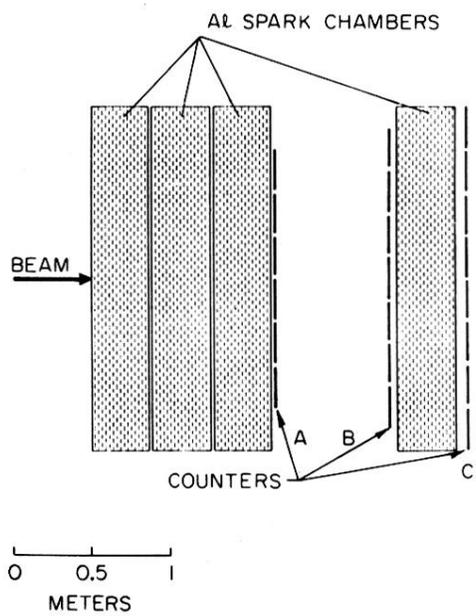
FIG. 3. Schematic of the detector showing the optical spark chambers and scintillation counters. Each of the four spark-chamber modules consisted of eleven 2.5-cm-thick aluminum plates.
