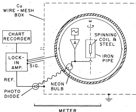
FIG. 2. Schematic of the apparatus. The signal from the oscillator is amplified (A) and applied by brushes to a spinning solenoid having a steel core.
