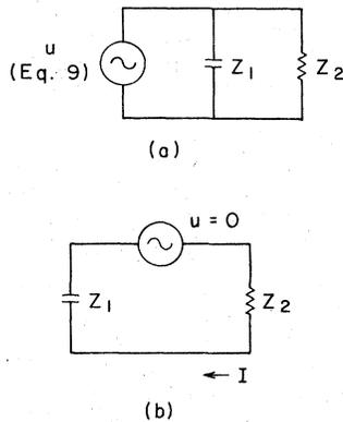
FIG. 4. Equivalent circuit of present experiment (a) using our hypotheses; (b) using Djurić's (Ref. 12).
