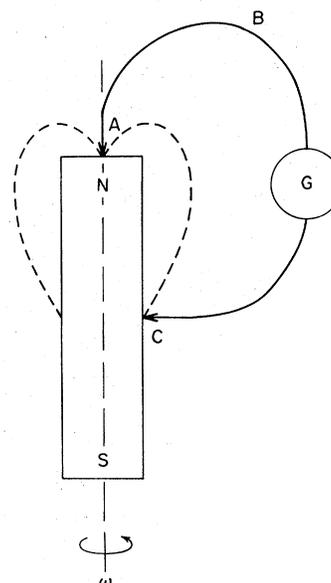
FIG. 1. Faraday's unipolar generator. A spinning magnet generates a current in the stationary wire ABC. The driving emf is proportional to the magnetic flux through the dashed surface.
