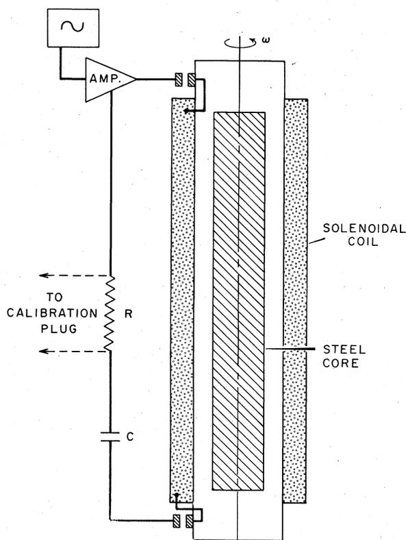
FIG. 3. Detail of spinning solenoid and steel core.
