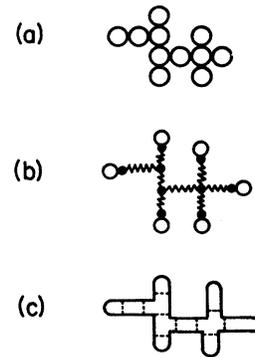
FIG. 2. (a) A typical vacuum graph that occurs in the Hartree approximation for theories with four-field interactions. These are characterized by bubbles hooked together to form trees. (b) Summing the chains of bubbles can form bound states denoted by wavy lines. (c) Corresponding graph in the generalization of the Hartree approximation to theories with trilinear interactions. This also has the bound-state structure (b) arising from a ladder sum.
