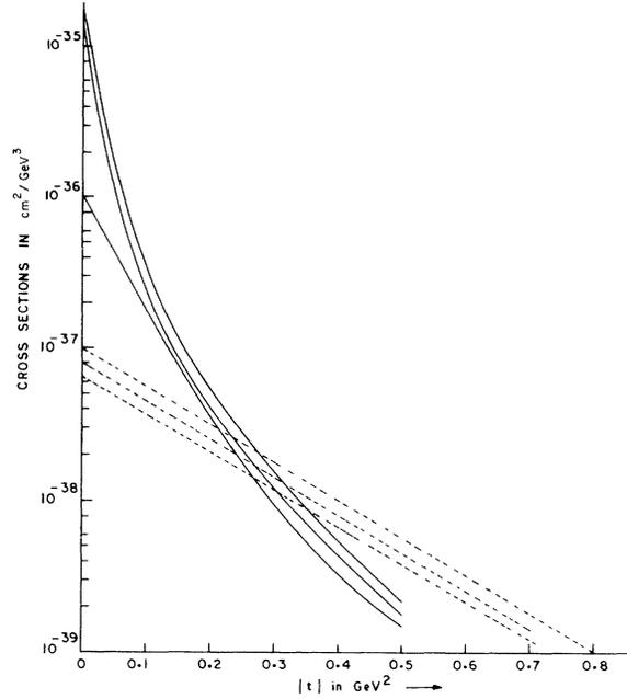
FIG. 2. Dashed lines are the inclusive cross section  $E_D(d\sigma/d\Omega' dE' d^3k)$  for  $\nu + p \rightarrow \mu^- + D^+ + X$ , for  $s = 80, 100$ , and  $120 \text{ GeV}^2$ . Solid curves are for the diffractive process  $\nu + p \rightarrow \mu^- + D^{*+} + p$  for above values of  $s$ .
