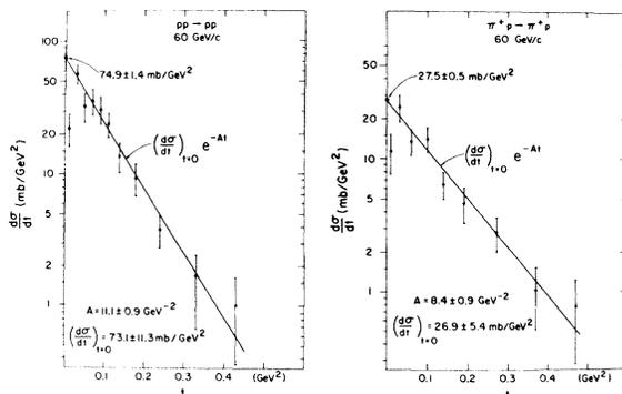
FIG. 1. Elastic-scattering distributions for  $\pi^+p$  and  $pp$  channels at 60 GeV/c. The stars at  $t=0$  indicate the values for  $d\sigma/dt$  expected from the optical theorem. The values for  $A$  and  $(d\sigma/dt)_{t=0}$  are from fits to the data.
