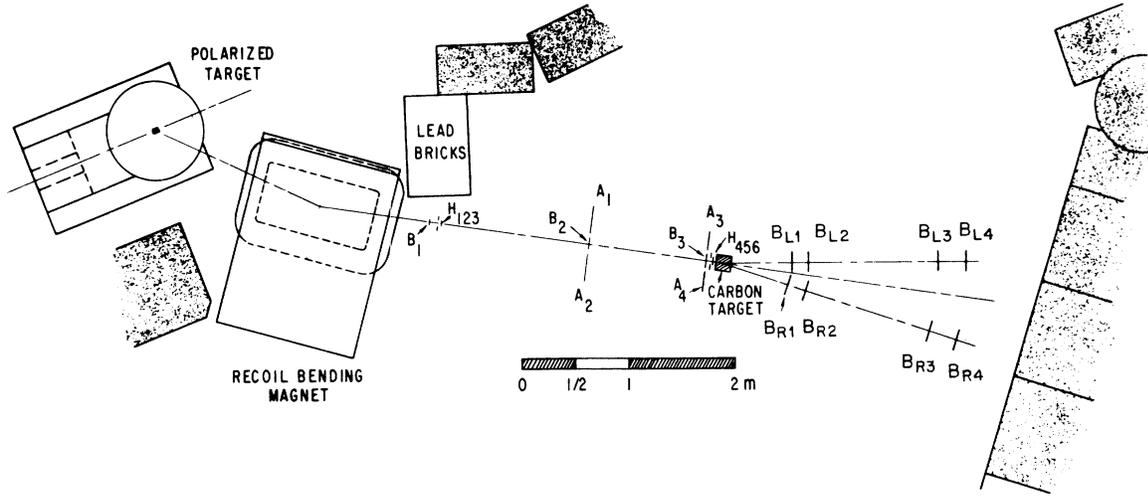
FIG. 1. Layout of the recoil ( $B$ ) arm and the  $B$  polarimeter. The recoil proton is momentum-analyzed by the recoil magnet and then detected by the  $B_1 B_2 B_3$  counters. The  $H_{123}$  and  $H_{456}$  hodoscopes monitor its angle and position prior to its scattering from the carbon target, while the  $B_L$  and  $B_R$  telescopes detect the  $p$ -C scattering to the left and the right. The  $A$  counters reduce background.
