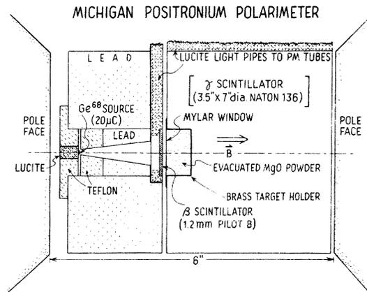
FIG. 1. Polarimeter apparatus, shown in cross section, has cylindrical symmetry. Positrons from  $^{68}\text{Ge}$ - $^{68}\text{Ga}$  source form positronium in the MgO target, and decays are detected by the  $\gamma$  scintillator.
