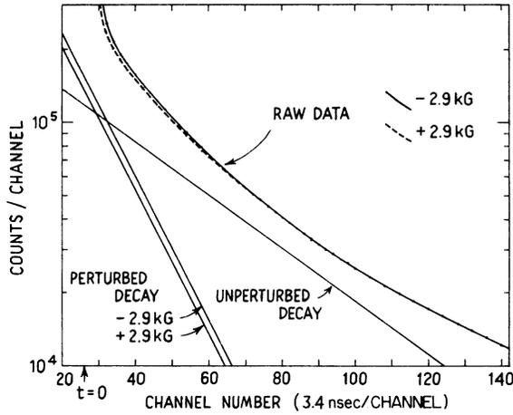
FIG. 2. Raw Ps decay data. The components were found by a computer fit. The asymmetry is given by the difference in count rates in early channels, labeled perturbed decay, when  $\vec{B}$  is reversed.
