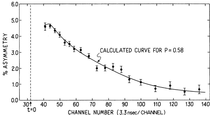
FIG. 3. Measured asymmetry at  $B = 2.9$  kG. Statistical errors are shown.
