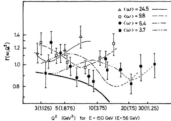
FIG. 5. The experimental data of  $r(\omega, Q^2)$  defined by (4.1). Narrow lines show the result of the formula (2.3). A bold line represents the values for the formula  $r^{01}(\omega, Q^2) = F_2^{01}(\omega, Q^2) / F_2^{01}(\omega, Q_0^2)$ , where  $F_2^{01}(\omega, Q^2) = (1 + Q^2/\Lambda^2)^{-2} \mathcal{F}_2(\omega)$  and  $Q_0^2 = 3Q^2/8$ .
