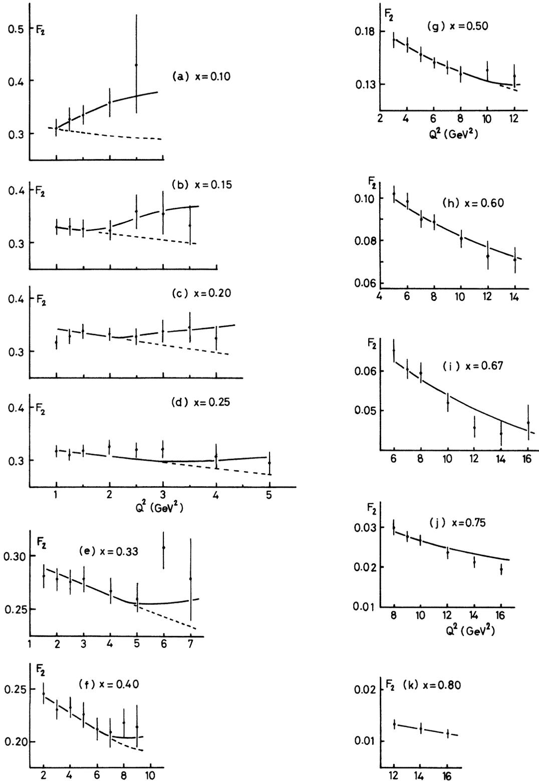
FIG. 2. The experimental values of  $F_2(\omega, Q^2)$  for a proton target versus  $Q^2$  for fixed values of  $x$ . The solid lines are resulting plots of the formula (2.3), which is discussed in Sec. IV. The dashed lines represent plots of the values of  $F_2^{\text{el}}(\omega, Q^2)$ , where  $F_2^{\text{el}}(\omega, Q^2) = (1 + Q^2/\Lambda^2)^{-2} \mathcal{F}_2(\omega)$  with  $\Lambda^2 = 50 \text{ GeV}^2$ .
