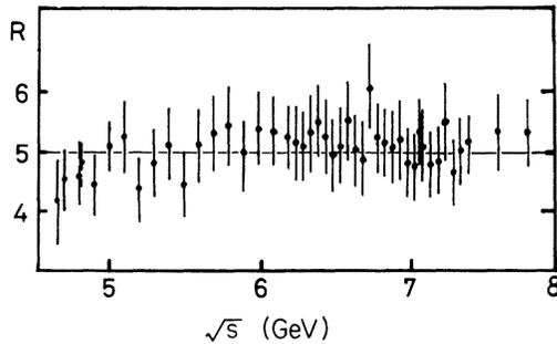
FIG. 3. The experimental data of  $R = \sigma(e^+e^- \rightarrow \text{hadrons}) / (4\pi\alpha^2/3s)$ .
