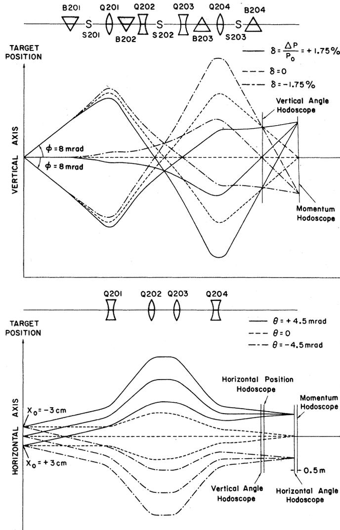
FIG. 4. Calculated trajectories through the spectrometer for selected initial values of horizontal and vertical angles ( $\theta$  and  $\phi$ ), horizontal position ( $x$ ), and momentum deviation ( $\delta$ ).
