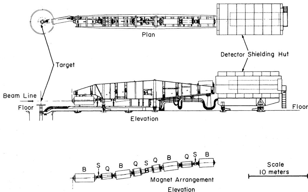
FIG. 3. Plan and elevation views of the SLAC 20-GeV/c spectrometer. The magnet arrangement is shown at the bottom of the figure with the symbols *B*, *Q*, and *S* representing dipole, quadrupole, and sextupole magnets, respectively.
