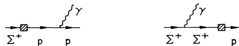
FIG. 1. Pole-model diagrams relevant for the decay \Sigma^+ \rightarrow p \gamma . The shaded box represents the weak Hamiltonian.
