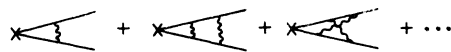
FIG. 7. The graphs which contribute to the renormalization of \Gamma_S(p, p, 0) in massless fermion QED.
