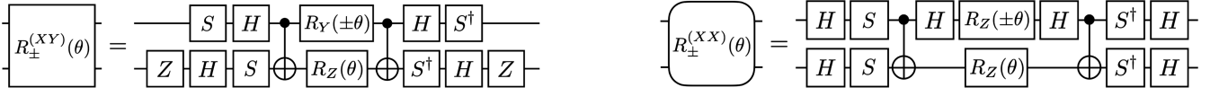
FIG. 5. Circuits implementing R_{\pm}^{(XY)}(\theta) = \exp[-i\frac{\theta}{2}(\hat{Y}\hat{X} \pm \hat{X}\hat{Y})] (left) and R_{\pm}^{(XX)}(\theta) = \exp[-i\frac{\theta}{2}(\hat{X}\hat{X} \pm \hat{Y}\hat{Y})] (right).
