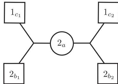
FIG. 3. Quiver diagram for SU(2) SQCD with four fundamental chirals. In the diagram, a circle node represents a gauge group and square nodes denote flavor groups. The number  $N$  within a node means SU( $N$ ) for  $N > 1$  and U(1) for  $N = 1$ .
