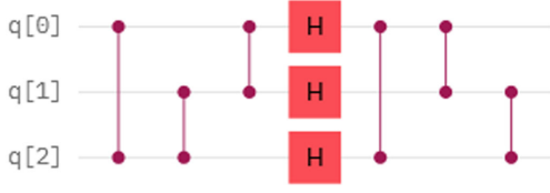
FIG. 6. The scrambling unitary operator used to realize the quantum computation. The scrambling unitary is composed by six controlled-Z gates and three Hadamard gates. The ordering of the left or the right three controlled-Z gates does affect the scrambling unitary.
