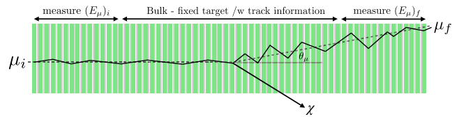
FIG. 1. A sketch of a muon track at FASER \nu . The initial and final energies can be estimated using the MCS method, where we emphasize using the solid black lines that the MCS angles would generically increase after the muon losses energy. In practice, the MCS angles are \mathcal{O}(1 \text{ mrad}) and the muon tracks appear as straight lines (dashed).
