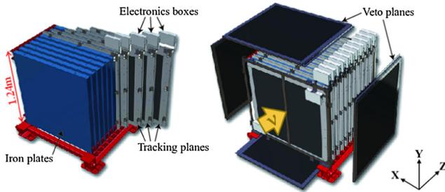
FIG. 4. An exploded view of a standard module.
