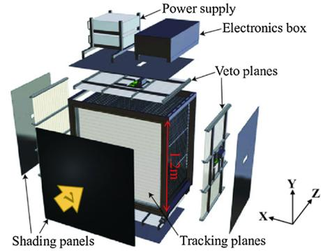
FIG. 6. An exploded view of the proton module.
