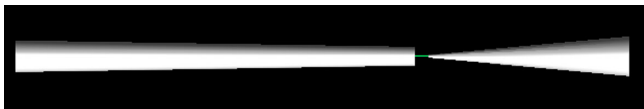
FIG. 5. Model of the best antenna design, individual 8, evolved in generation 23. This bicone is shown on its side here, with the top side on the left. Other individuals are not shown because they are not visually distinguishable from this one.
