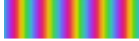
FIG. 1. An abs-arg plot of a plane wave demonstrating its linear phase profile.
