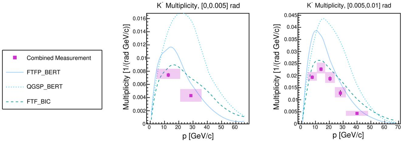
FIG. 22. Combined multiplicity measurements for  $K^-$  analysis. Error bars denote statistical uncertainty, and total systematic uncertainty is shown as a shaded band. Results are compared to three Monte Carlo models. Two representative angular bins are shown.
