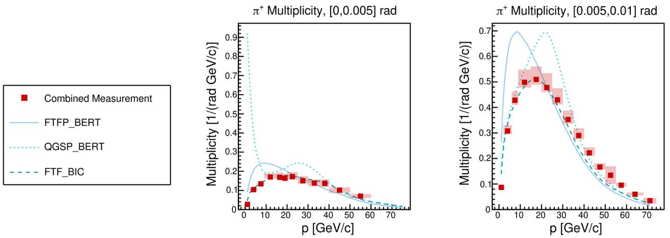
FIG. 17. Combined multiplicity measurements for  $\pi^+$  analysis. Error bars denote statistical uncertainty, and total systematic uncertainty is shown as a shaded band. Results are compared to three Monte Carlo models. Two representative angular bins are shown.
