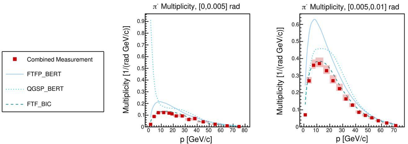
FIG. 18. Combined multiplicity measurements for  $\pi^-$  analysis. Error bars denote statistical uncertainty, and total systematic uncertainty is shown as a shaded band. Results are compared to three Monte Carlo models. Two representative angular bins are shown.
