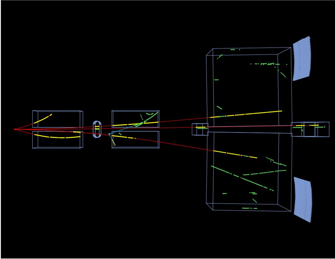
FIG. 3. Reconstructed event from the 2017 120 GeV/ $c$  proton-carbon dataset. Event was reconstructed using the SHINE-native reconstruction chain. A forward-going track spanning the GTPC and all three FTPCs can be seen. Yellow points and red lines represent TPC point measurements associated with vertex tracks. Green points represent TPC point measurements associated with out-of-time beam particles or tracks produced by out-of-time beam particles.
