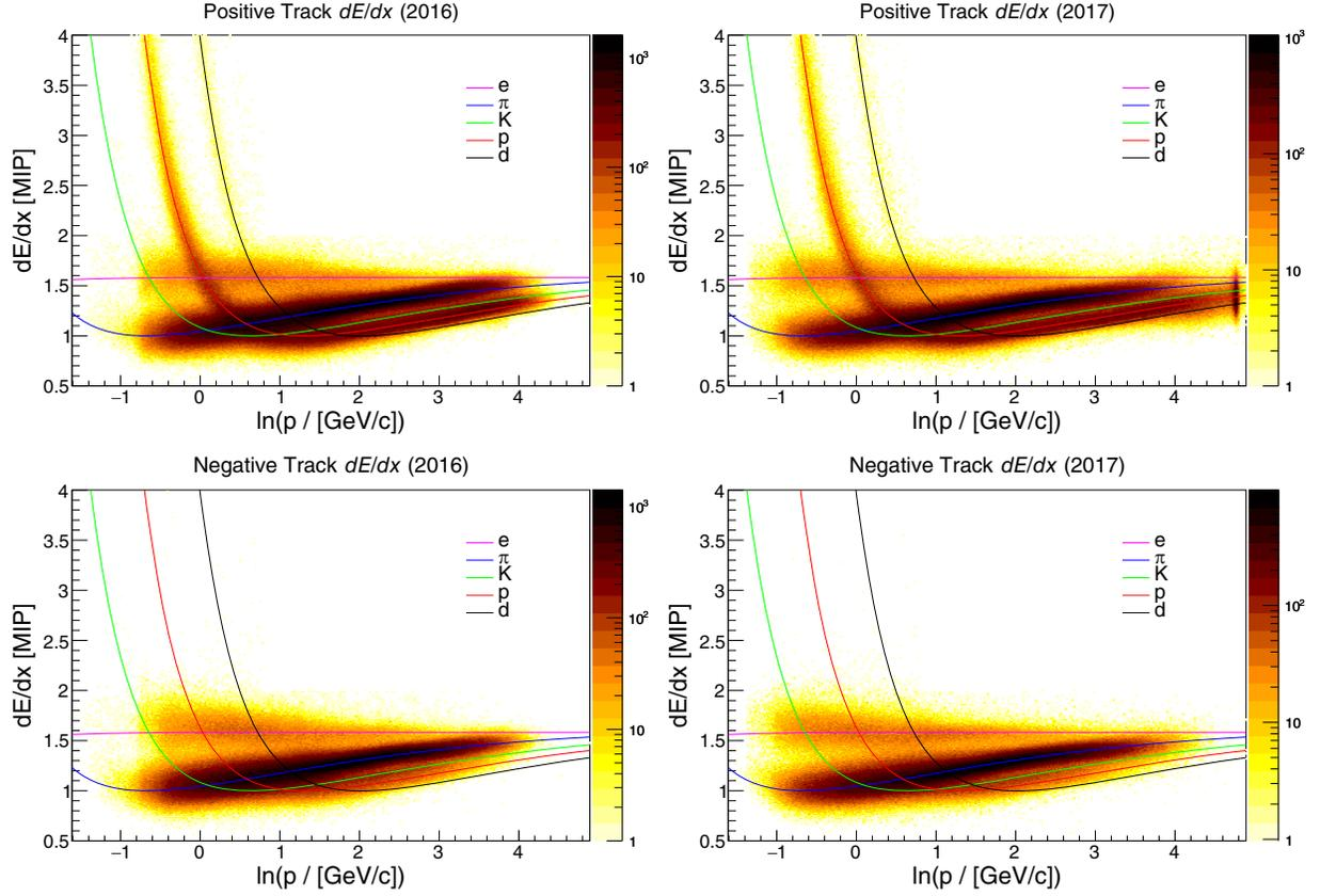
FIG. 4. Two-dimensional distributions of charged track  $dE/dx$  vs.  $\ln(p)$  for the 2016 and 2017 datasets after applying track quality cuts. The lines represent Bethe–Bloch predictions for various particle species. Increased acceptance in the 2017 dataset is visible in the extension of the distribution to lower total momenta (due to a lower magnetic field setting) and a prominent peak in positively charged track  $dE/dx$  at the beam momentum ( $\ln(p)/[\text{GeV}/c] = 4.78$ ).
