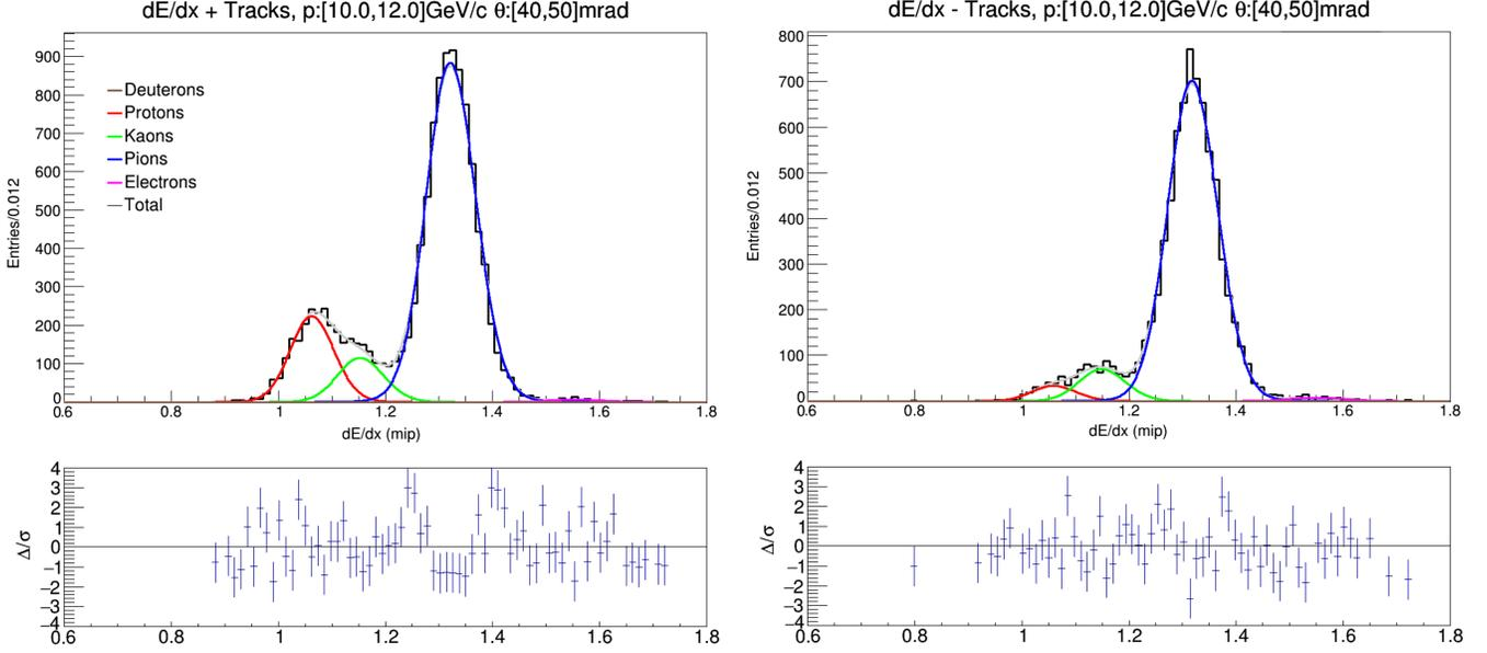
FIG. 5. Example  $dE/dx$  distribution fit for one kinematic bin showing positively (left) and negatively (right) charged track distributions. This kinematic bin shows an abundance of pions in both the positively and negatively charged track distributions, a significant fraction of protons, and a lack of antiprotons. This is characteristic of the 120 GeV/c proton-carbon reaction.
