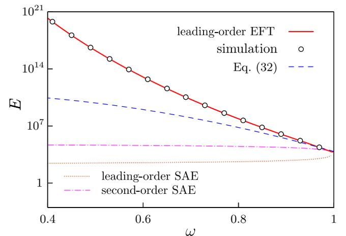
FIG. 8. The energy  $E(\omega)$  of three-dimensional monodromy oscillons at  $p = 0.95$  and  $\varepsilon = 0.05$ .
