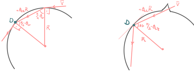
FIG. 5. Left: for a perfectly spherical Earth, the antineutrinos entering the Earth and hit the detector at D from below the surface can only be refracted at a maximum angle of \frac{\pi}{2} - \theta_{\text{cr}} , so there is essentially no possibility of reflection at the position of the detector. This maximally refracted \bar{\nu} s come from a distance of \mathcal{O}(\theta_{\text{cr}} R_{\oplus}) \sim 1 km. Right: for an imperfect Earth, the presence of a mountain can allow for antineutrino rays to enter the Earth and hit D at an angle larger than critical, so reflection is now possible.
