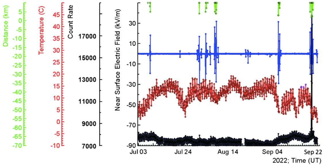
FIG. 1. Summer 2022: black—time series of 1-min count rates of STAND3 plastic scintillator of 1 m<sup>2</sup> area and 3 cm thickness; blue—disturbances of the NSEF measured by EFM 100 electric mills produced by the BOLTEK firm, widely used in atmospheric physics research; red—outside temperature; green—distances to lightning flashes.
