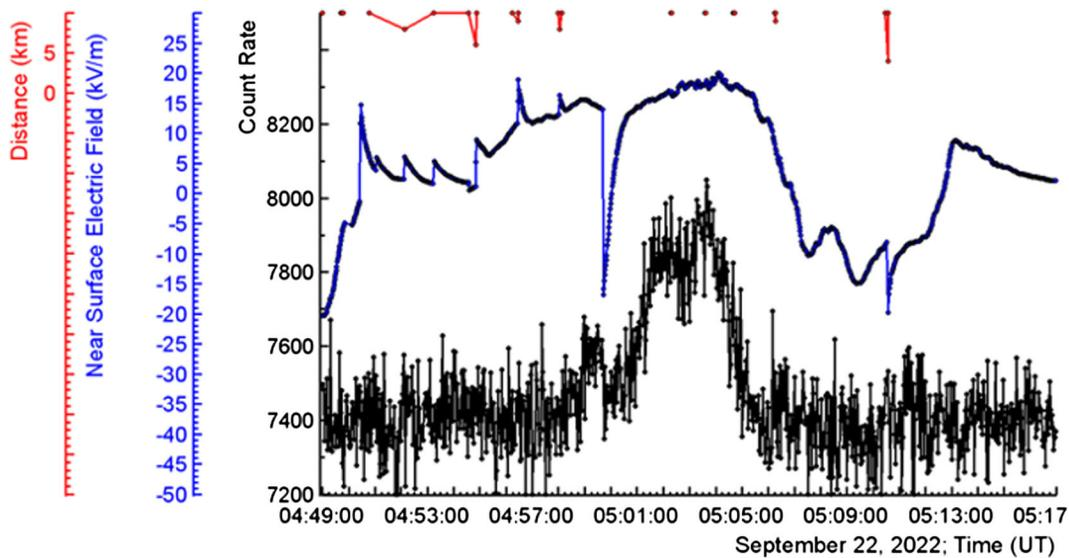
FIG. 17. Time series of 2 s count rates of ASNT scintillator of 4 m<sup>2</sup> area and 60 cm thickness, black; disturbances of the NSEF, blue; distances to lightning flashes, red.
