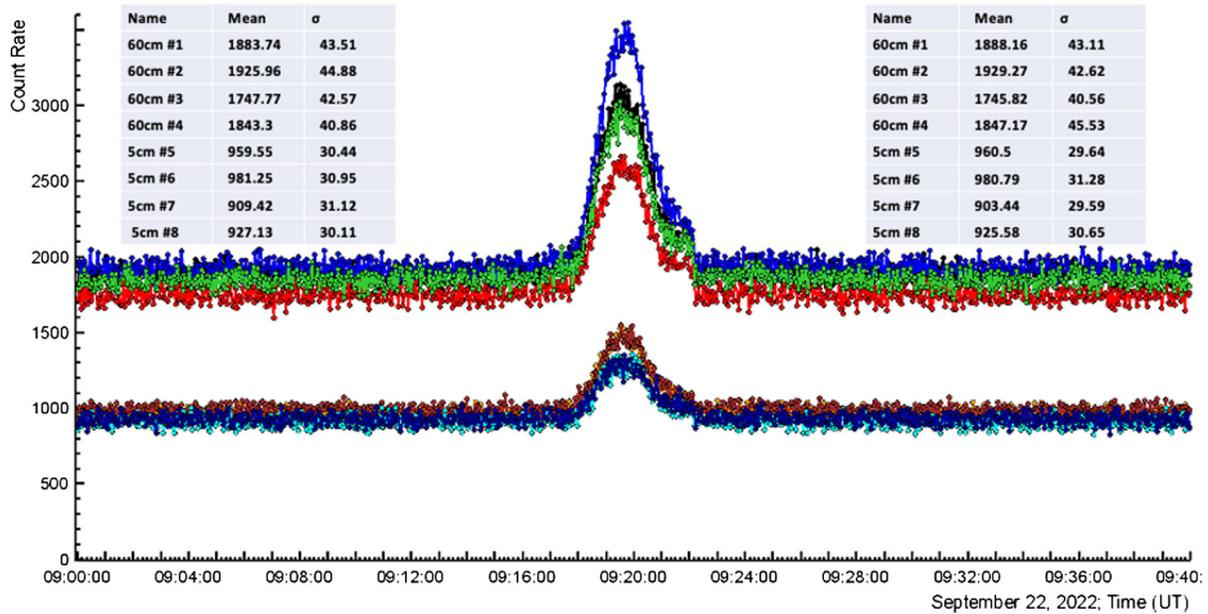
FIG. 3. 2 s time series of count rates of 8 ASNT scintillators (four 5 cm thick “veto” scintillators and four 60 cm thick spectrometric scintillators). The insets show mean values and variances of the count rates before and after TGE.
