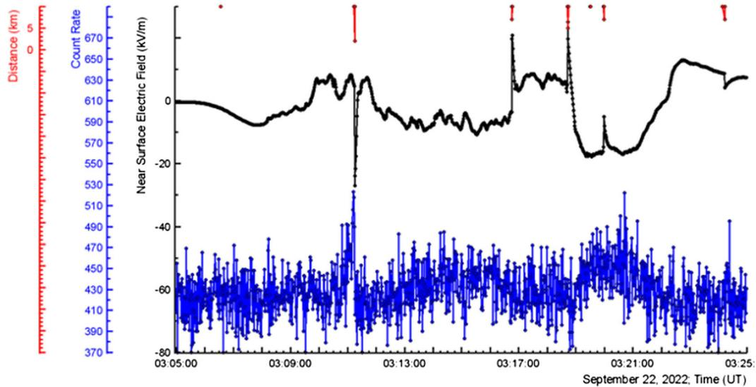
FIG. 15. Disturbances of the NSEF, black; time series of 1 s count rates of STAND1 plastic scintillator of 1 m<sup>2</sup> area and 1 cm thickness, blue; distances to lightning flashes, red.
