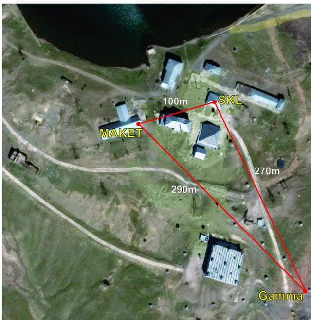
FIG. 22. STAND1 detector network. Each of the three units comprises vertically stacked three 1 cm thick and 1 m<sup>2</sup> area plastic scintillators and the same area stand-alone 3 cm thick plastic scintillator.
