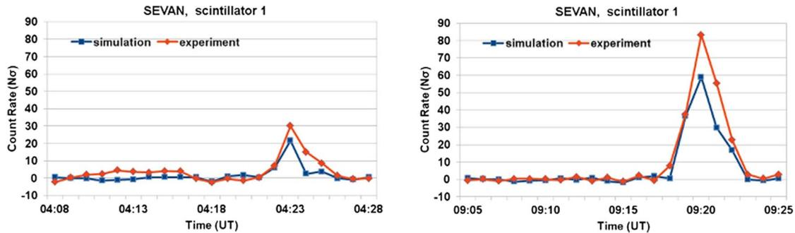
FIG. 21. Comparison of count rates measured by upper scintillator of SEVAN detector with calculated ones recovered by ASNT.
