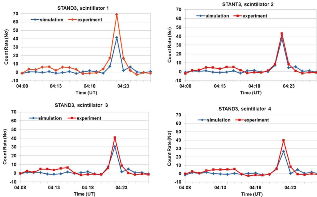
FIG. 20. Comparison of count rates measured by four stacked scintillators of STAND3 detector with calculated ones recovered by ASNT (minutes from 4:21–4:23).
