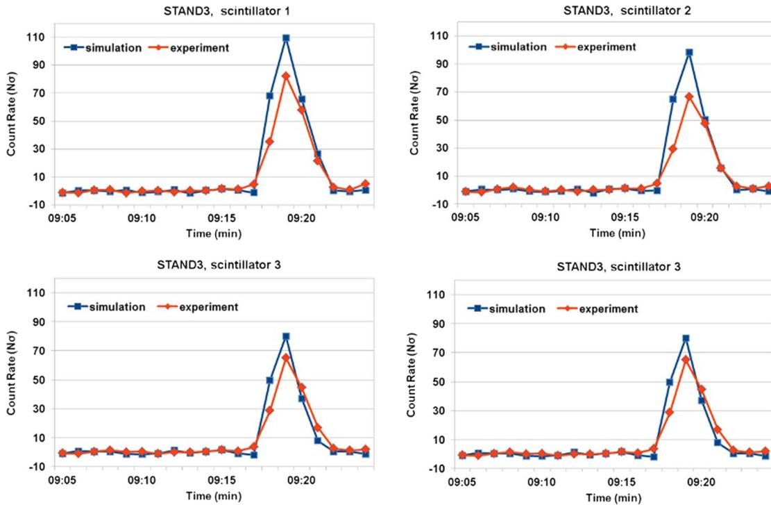
FIG. 19. Comparison of count rates measured by four stacked scintillators of STAND3 detector with calculated ones recovered by ASNT (minutes from 9:17 to 9:21).
