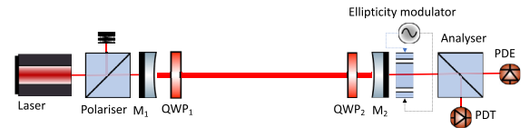
FIG. 2. The proposed polarimetry scheme for sensing the coupling of the axion field to photons by using a Fabry-Pérot cavity and two quarter-wave plates (QWP 1 and QWP 2 ). PDT/PDE are the photodiodes in the transmission and in the extinction port of the analyzer, respectively, and M 1 /M 2 are mirrors that delimit the Fabry-Pérot cavity.
