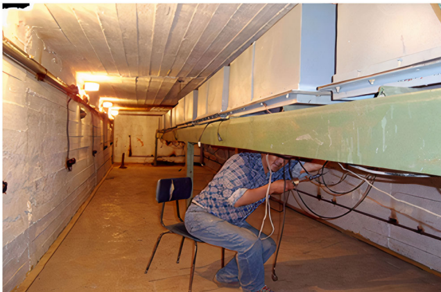
FIG. 2. Muon detector with total area of 20 \text{ m}^2 for registering muons with a threshold \epsilon_{\text{thr}} \geq 1 \text{ GeV} .
