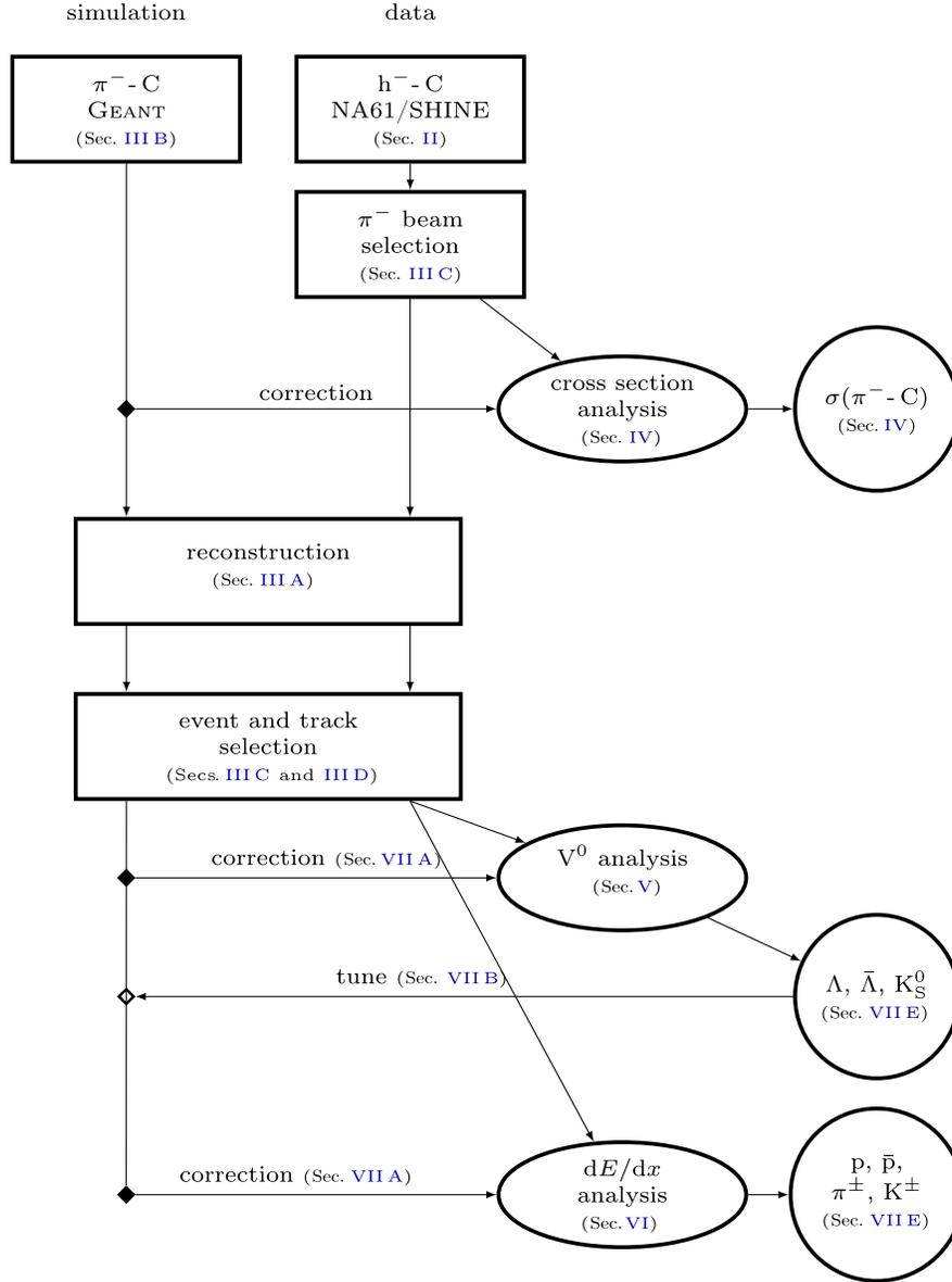
FIG. 1. Schematic view of the analysis presented in this paper.
