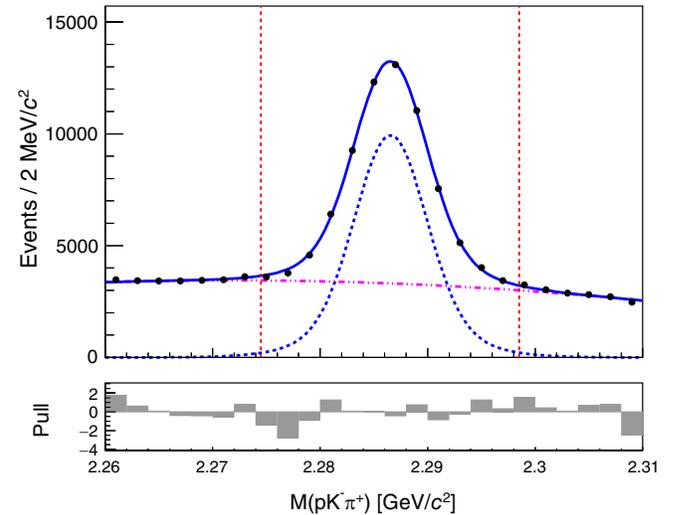
FIG. 3. Fit to the invariant mass distribution of  $\Lambda_c^+$  in data. The solid blue curve shows the best fitted result, the dashed blue curve shows the signal component, and the dot-dashed purple curve shows the fitted backgrounds. The red dashed lines show the defined  $\Lambda_c^+$  signal region.
