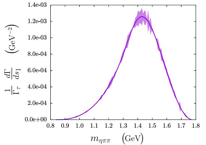
FIG. 2. Invariant mass spectrum of the  $\tau^- \rightarrow \eta\pi^-\pi^0\nu_\tau$  transition. The purple stripe is the error band obtained from the Gaussian variation of parameters at each bin, the solid purple line represents the mean of the distribution.
