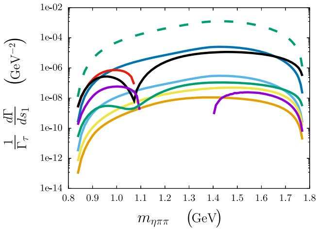
FIG. 5. Different contributions to the differential decay width, shown in a logarithmic scale. Because of this, some of them cannot be shown in this figure, since interference terms are negative in certain regions of the invariant mass range. The color code follows: pure SM (dark green), SM-V (dark blue), SM-A (red), SM-T (black), A-V (lilac), V-T (green), A-T (purple),  $|V|^2$  (pale blue),  $|A|^2$  (yellow),  $|T|^2$  (orange).
