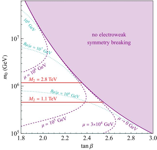
FIG. 1. Contours of  $\mu$  (purple),  $M_2$  (red), and  $B\mu/\mu$  (cyan), where the gaugino masses are set by AMSB at high scale and  $\mu$  is set as needed for EW symmetry breaking, assuming  $m_{H_u}$  and  $m_{H_d}$  are  $m_0$  at the GUT scale. EW symmetry is unbroken in the purple shaded region. The contour with  $\mu = 1.1$  TeV, of interest for dark matter, is indistinguishable from the  $\mu \rightarrow 0$  boundary, see text for details.
