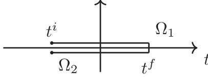
FIG. 3. Representation of the Schwinger-Keldysh path. The small vertical line at  $t_f$  does not contribute to the path integral. Phase-space variables in the upper contour and lower contour are labeled as  $w_1$  and  $w_2$ , respectively.
