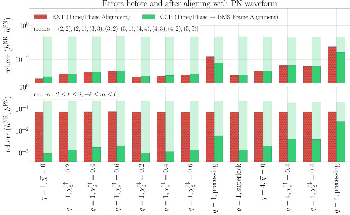
FIG. 3. Comparison of the relative error between a CCE waveform and a PN waveform (green) to the relative error between an extrapolated waveform and a PN waveform (red). The relative error is computed over a three-orbit window that begins at 1200M past the initial time of the simulation. For the CCE waveforms, we show two errors: one where the error is computed when the time and phase freedom is fixed (faint) and one where the error is computed when the BMS freedom is fixed (full). With the extrapolated waveforms, we only fix the time and phase freedom. The top panel shows the relative error when only the (2,2), (2,1), (3,3), (3,2), (3,1), (4,4), (4,3), (4,2), and (5,5) modes are included, while the bottom panel shows the error when every mode up to \ell = 8 is included. These simulations correspond to those found in Table I.
