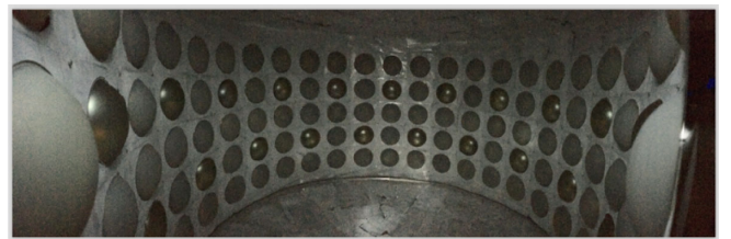
FIG. 6. The inside of the CCM120 detector. The 120 inner PMTs are placed around the cylinder barrel, 96 coated, 24 uncoated, and TPB painted reflective foils are also shown.
