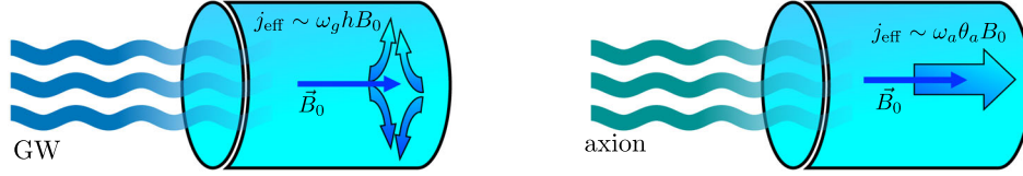
FIG. 1. A cartoon illustrating the differences between (left) GW-EM conversion and (right) axion-EM conversion in the presence of an external magnetic field \mathbf{B}_0 . The GW effective current is proportional to \omega_g h B_0 , with a direction dependent on the GW polarization and a typical quadrupole pattern, yielding a signal field with amplitude h B_0 . The axion effective current is proportional to \omega_a \theta_a B_0 , with a direction parallel to the external field \mathbf{B}_0 , yielding a signal field with amplitude \theta_a B_0 . The differing geometry of the effective current yields different selection rules for coupling the GW and axion to cavity modes.
