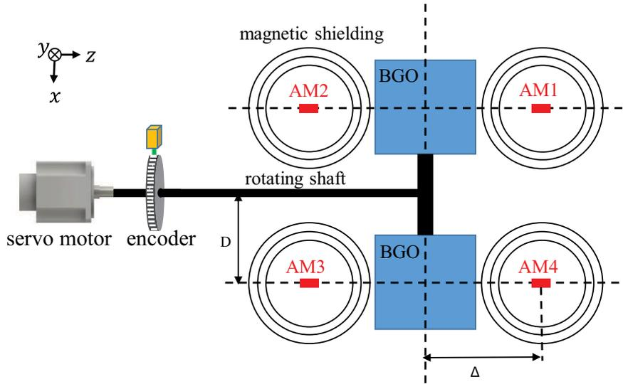
FIG. 1. Schematic of the proposed experiment. The servo motor rotates two dense, nonmagnetic cylinder source masses with frequency  $\omega_0$ , inducing pseudomagnetic field signals to the surrounding AMs if exotic spin-dependent interactions exist. The encoder monitors the rotating angle and frequency in real-time.
