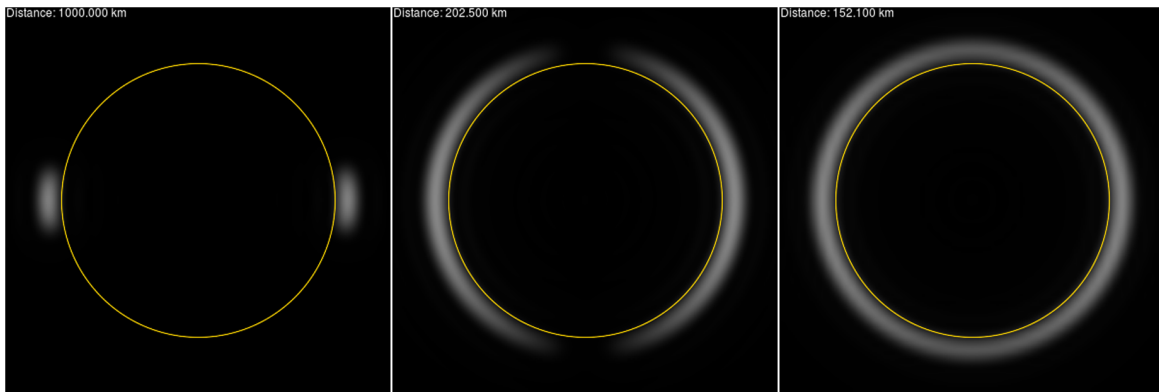
FIG. 5. View of a distant star by a telescope approaching the SGL optical axis, at distances of 1,000 km, \sim 200 km and \sim 150 km. The geometric projection of the star to the image plane would yield a disk with a radius of 200 km. As the imaging telescope approaches this distance, a full Einstein-ring forms; subsequently, the ring brightens and becomes uniform as the telescope settles on the optical axis.
