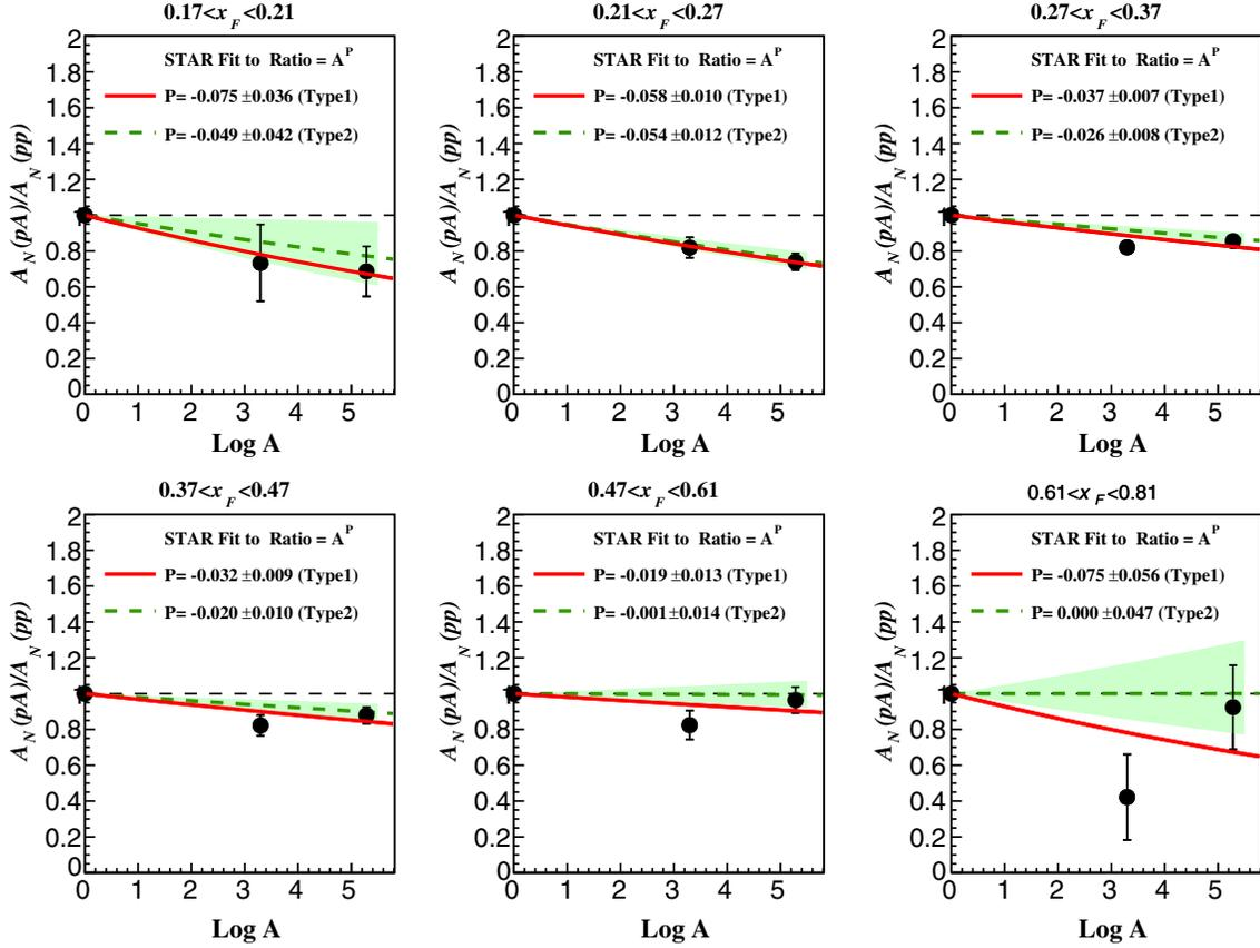
FIG. 8. The ratio of  $A_N$  for  $pA$  scattering to that for  $pp$  scattering is shown for six  $x_F$  regions, averaging over the full range of  $p_T$  dependence. The fitted form for these ratios as a function of  $A$  is obtained using type 1 and type 2 analyses as described in the text. The dependence of  $A_N$  as a function of  $\log A$  is displayed with a filled error band, obtained from the type 2 analysis, shown as the dashed line.
