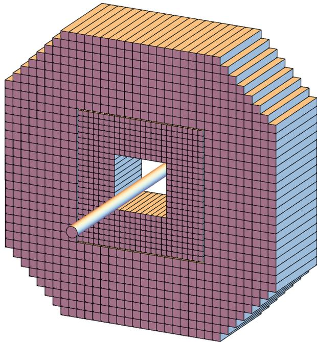
FIG. 1. The layout for the FMS calorimeter around the RHIC beam line located about seven meters west of the nominal STAR interaction point. The FMS consists of lead glass blocks with lengths corresponding to 18 radiation lengths. There are 788 outer blocks with front face dimensions of  $5.8 \times 5.8$  cm. and 476 inner blocks with front face dimensions of  $3.8 \times 3.8$  cm.
