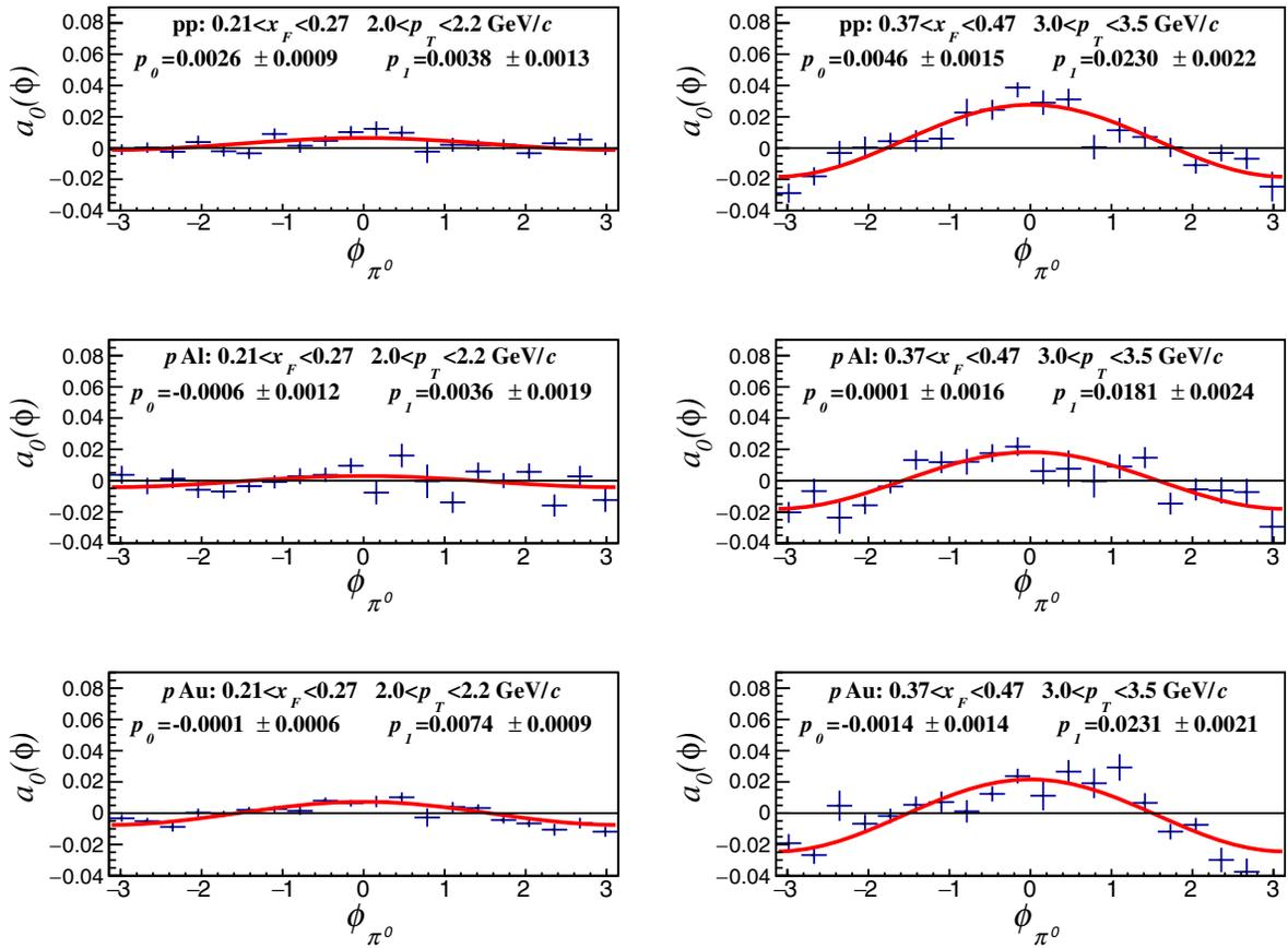
FIG. 3. Uncorrected transverse spin asymmetries for the same six kinematic regions as in Fig. 2. The azimuthal  $\phi_{\pi^0}$  distributions of the uncorrected asymmetries,  $a_0(\phi)$ , are shown for events in the mass range  $0.015 < M_{\gamma\gamma} < 0.255 \text{ GeV}/c^2$ . Fits to the functional form from Eq. (6) are shown with fitted parameter values  $p_0$  and  $p_1$ .
