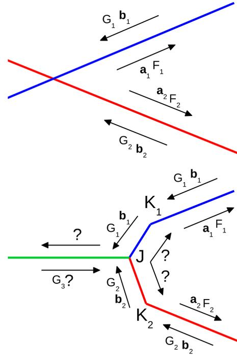
FIG. 6. Schematic picture of left- and right-moving modes of elastic transonic strings for the gauge described in the main text, Sec. II. The upper panel shows left- and right-moving modes before the collision of strings, and the lower panel shows modes after. Moving modes with question symbol should be determined by equations for Y junction (31) and (32).
