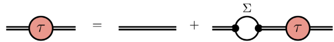
FIG. 3. A diagrammatic depiction of the isobar propagator from Eqs. (4) and (5), representing the resummation of \pi\pi interactions within the isobar to all orders. Double and single lines denote the isobar and stable particle propagators, respectively.
