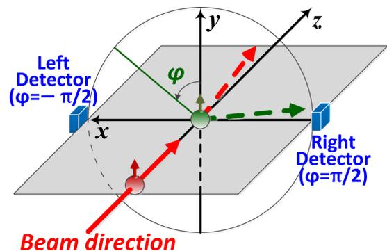
FIG. 1. A schematic view of the  $p^\uparrow p^\uparrow$  spin correlated asymmetry measurements at HJET. The recoil protons are counted in left/right symmetric detectors. The beam moves along the  $z$  axis. The transverse polarization direction is along the  $y$  axis.
