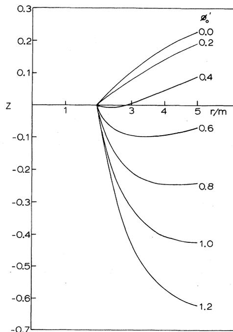
FIG. 3. Frequency shifts measured by an observer at  $r = 1.96m$  as a function of the radial coordinates of the sources and the initial value of  $\phi'$ .
