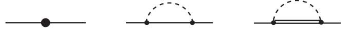
FIG. 2. Feynman diagrams which contribute to the nucleon self-energy up to order \epsilon^3 . Only nonvanishing diagrams are shown. Solid, dashed, and double lines represent nucleons, pions, and the \Delta , respectively. Solid dots (filled circles) denote leading-order (subleading and higher order) vertices from the effective Lagrangian.
