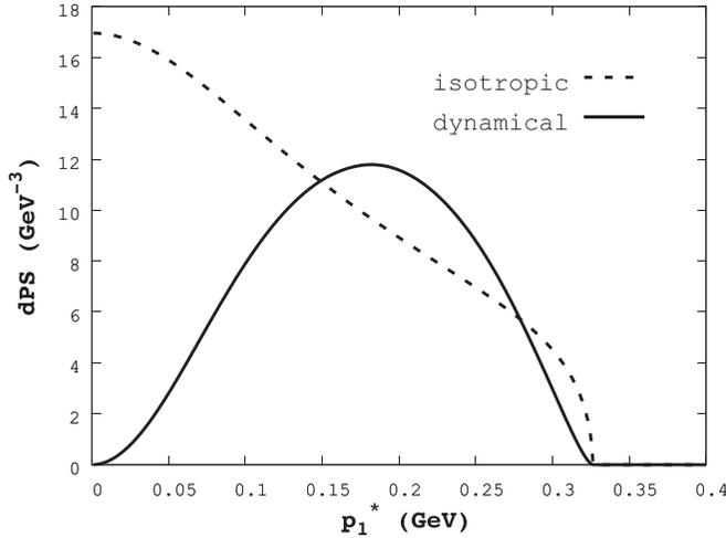
FIG. 1. Differential phase space function dPS calculated by Eq. (4) for the decay  $\omega \rightarrow 3\pi$ . Solid line corresponds to calculation with the full matrix element (19) while dashed line corresponds to result from the isotropic approximation.
