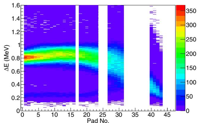
FIG. 3. Calibrated Bragg curve of the unscattered <sup>30</sup>S beam over the low-gain region of the active target. The depth of each pad is 4 mm with the beam penetration depth correlated with the pad number. Data from several pads are not shown for a variety of reasons; in general it was either because the electronics did not record a signal, or the energy deposit was arbitrarily lower than expected.
