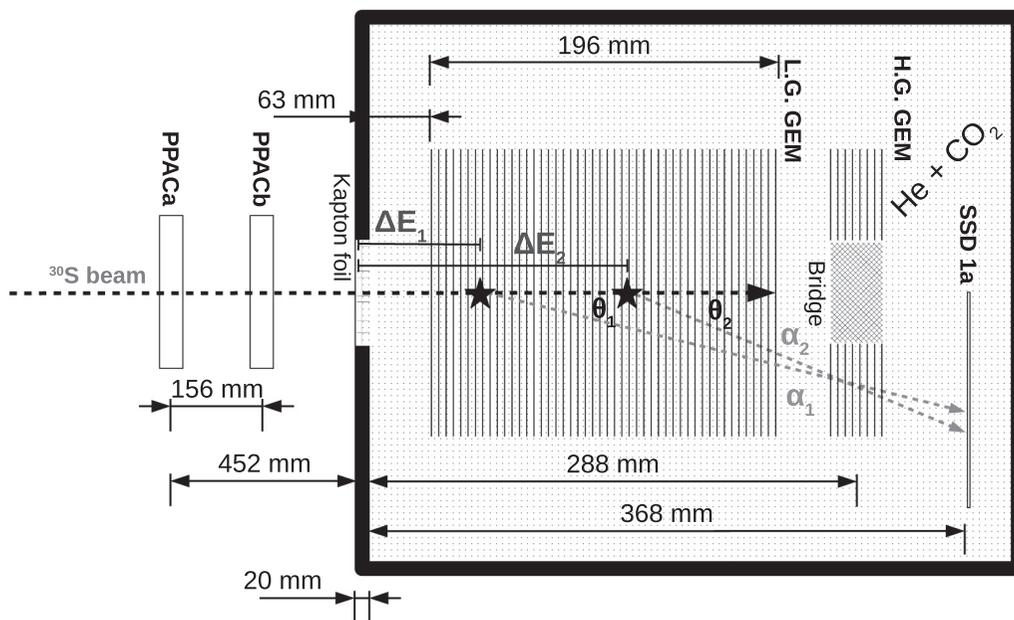
FIG. 2. Top-down cartoon of the experimental setup and the detectors used in the data analysis (not to scale—PPACs in particular are much further from the active target chamber than depicted). The differences between a higher energy scattering (denoted “ $\alpha_1$ ”) and a lower energy scattering (“ $\alpha_2$ ”) are shown.
