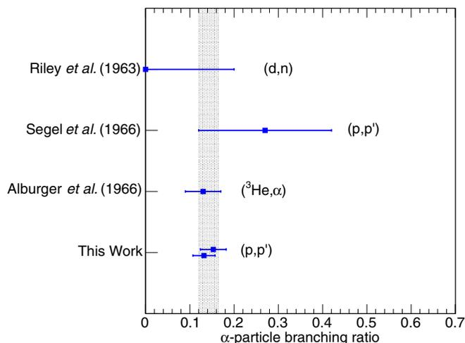
FIG. 7. Past and current results for the  $\alpha$ -particle branching ratio. The results for both methods used to determine the branching ratio in this work are shown. The gray band illustrates the new value for the branching ratio suggested in this work.
