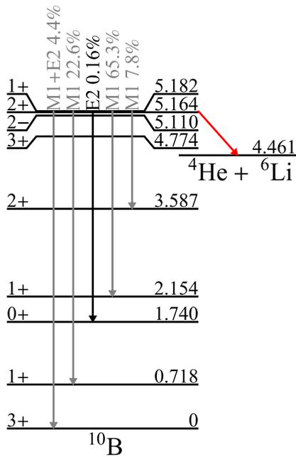
FIG. 1. Decay paths of the 5.164 MeV state. The pure  $E2$   $\gamma$ -ray transition to the  $T = 1$ ,  $J^\pi = 0^+$  state is shown in black, whereas  $M1$  and  $E2$  transitions to  $T = 0$  states are shown in gray. The transitions and energy levels are from Refs. [9,11].
